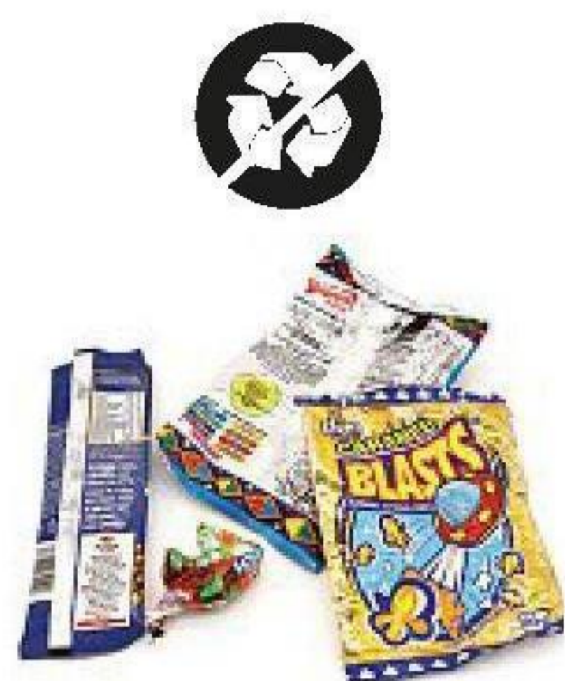
The packaging of snacks such as chocolate and snack bars, chip packets, sweet wrappers, biscuit wrappers – these are all multilayer laminates, in other words, layers of different plastics and foils “glued” together
